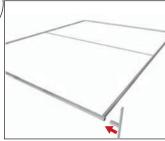
4. Connect feet to the frame by pressing & pushing.
