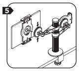
Press buttons,attach bracket, release buttons, and spin until you hear the click.
