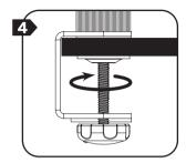
Turn the knobs on the C-clamps to secure the keyboard tray to your desk.
