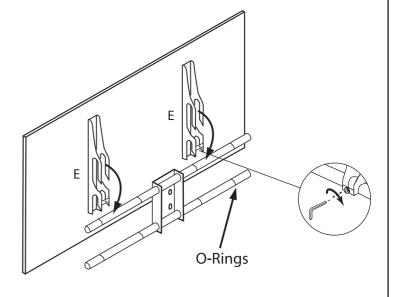
**Step 7.**Lift the LCD screen by 2 people and hook the brackets (E) on the Rail (C) as the picture shown. Check and make sure the LCD screen is centered. Tighten the bolts on Rail (C) and Brackets (E) by Allen key (F2) to secure the LCD screen to the Rails (C).
