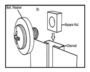
2. Slide the nut through the channel in the post. Tighten bolt at desired height.
