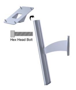
4. Screw the holder to the wall. Use the plastic wall plugs when securing to concrete.
