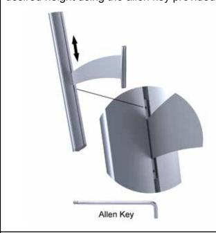
3. Secure the top bracket to the post with the bolts provided
