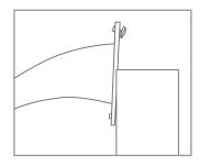
3. Assemble the iPad holder and loosely attach the included connector to the back of the plate to slide down the channel.
