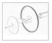
1. Connect the pole, base and weight as shown.
