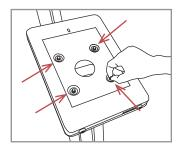
Before inserting the iPad, undo the 4 dome nuts on the inside of the iPad enclosure
