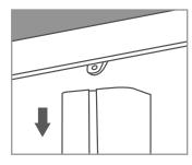
6. To attach the poster holder, slide the 2 connector plates down the channel of the pole to the desired height.
