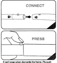
If can't snap when dismantle the frame, Pls push the tube forwardly, then push again.
