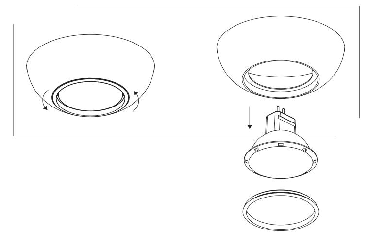
Place new LED in position and reverse the steps to connect the new LED.
