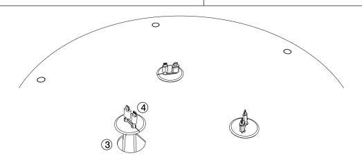
3 Remove cables from cable clip.
