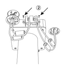
2 Unscrew the 2 screws on cable cover.
