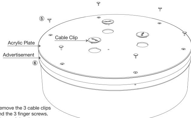
(5) Remove the 3 cable clips and the 3 finger screws.
