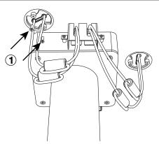
1 Detached the cable clip by unscrewing the 2 screws.
