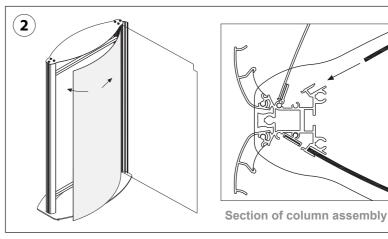
Place the full length plastic diffusion panel and clear plastic lens into the channels on the side columns (as shown in the detail drawing) ensuring that the decorative panel is at the bottom of the display
