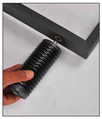
1. Screw in the spring feet to the metal frame.
