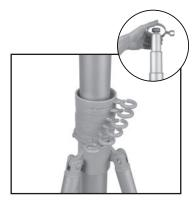
4. Slide all pole rings and locking clip over the telescopic pole
