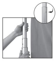
7. Extend the telescopic pole starting with the top section till the release button pop out.
