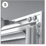
• Fix the frame to the wall through the four holes in the canal nearest to the corners.
