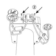
2 Unscrew the 2 screws on cable cover.
