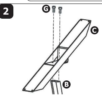
Attach mounting bracket to post using M8 socket head screws. Use supplied hex key.
