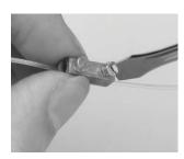
6. Slide the grip into desired position. Tighten the grip onto the wire using a screwdriver.
