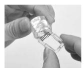
1. Release bottom of the ceiling fitting by squeezing the loop.
