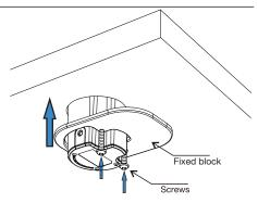
Position the fixed block underneath the MoQi and fix it with the screws provided.
