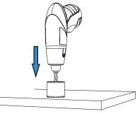
Drill holes with the wood drill in a flat positions.
