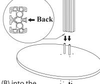
Step 2. Insert the Pole (B) into the support shafts (D), bottom fitted with M6 x 60mm screws by Allen key (H2)
