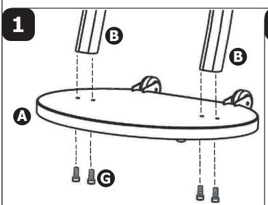
Attach posts to base using M8 socket head screws. Use supplied hex key.
