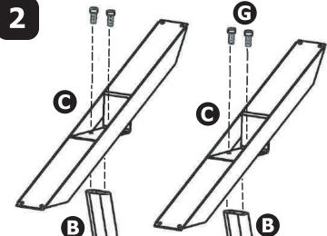
Attach mounting brackets to posts using M8 socket head screws. Use supplied hex key.
