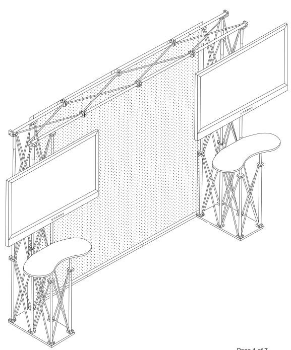
Thank you for purchasing our Display Center. This folding truss TV stand and display center is designed to accomodate two flat panel TVs from 32" up to 65" screen (diagonal) and weighing up to 36kg per TV. Assembly is easy with no additional tools required.
