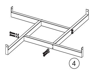
Step 2. Attach 3<sup>rd</sup> tube to 2<sup>nd</sup> tube with 2 Hex bolts.
