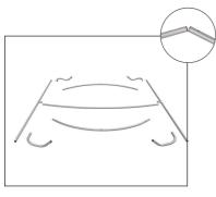
1. Assemble the two long curved and long straight sections.
