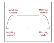
Connect corner sections to straight sections by matching the numbers.
