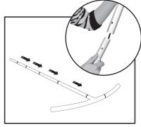
2. Assemble the straight pole and the curved top pole. Join together.
