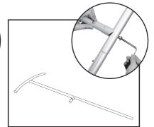
3. Insert shelf fitting in the middle of tube and tighten with an allen key.
