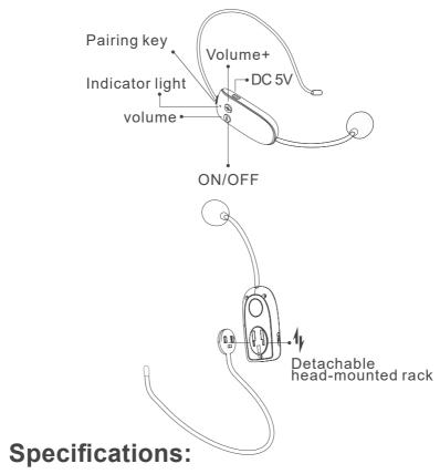
Microphone: Unidirectional condenser microphone
