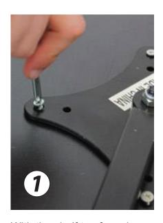
With the shelf top face down, place the flat bracket mount to the pre-drilled holes and fix them together with the short screws.
