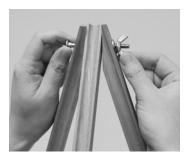
4. Thread the 2nd longest wing-nut and screw through all 3 legs at the top. The 2 angle cut legs rest flush against the back leg.
