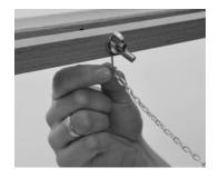
6. Screw the eyelet hook with chain to the tray.
